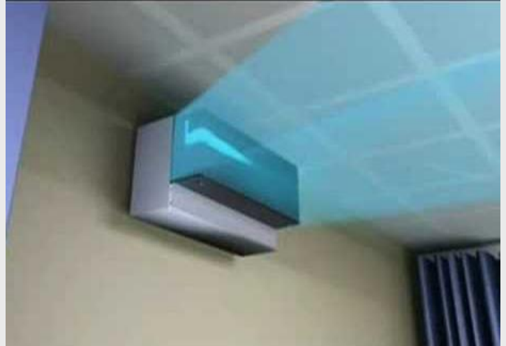
Figure 2 Room UVGI Units
